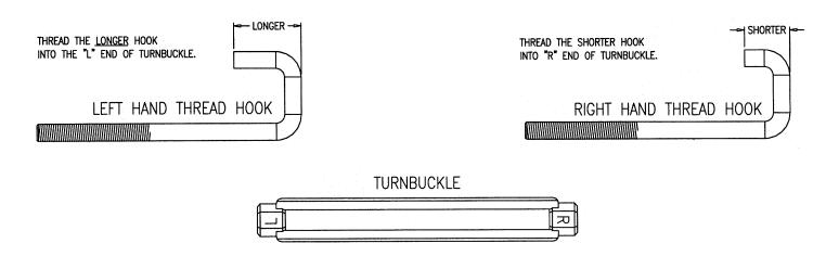
HOOKS MUST BE THREADED IN EQUALLY, APPROXIMATLY 1/4" INSIDE TURNBUCKLE
